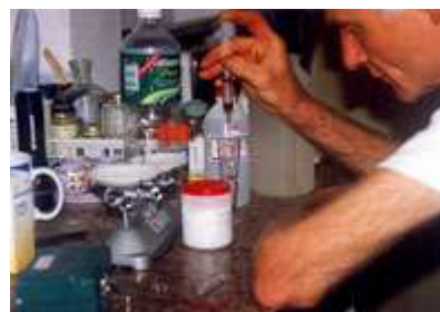
Keith checks the pH of the waste oil.
