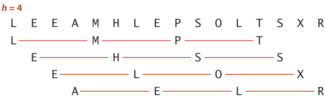
An h -sorted sequence is h interleaved sorted subsequences
