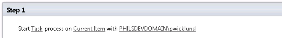
Figure 4.60 The Start Custom Task Process action has three parameters, the process instance, the item to start the task on, and the user(s) to assign the task to.
