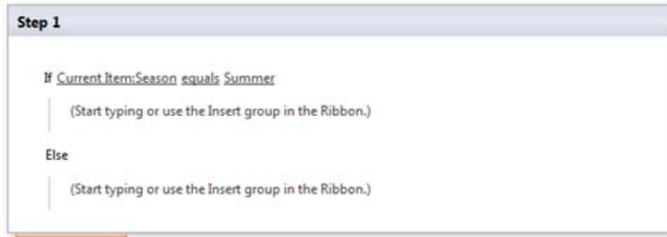
Figure 3.41 An Else-If branch added to a condition allows the workflow to perform specific processes whether the result of the condition is True or False. An Else without an additional condition will always be executed if the preceding If is false.
