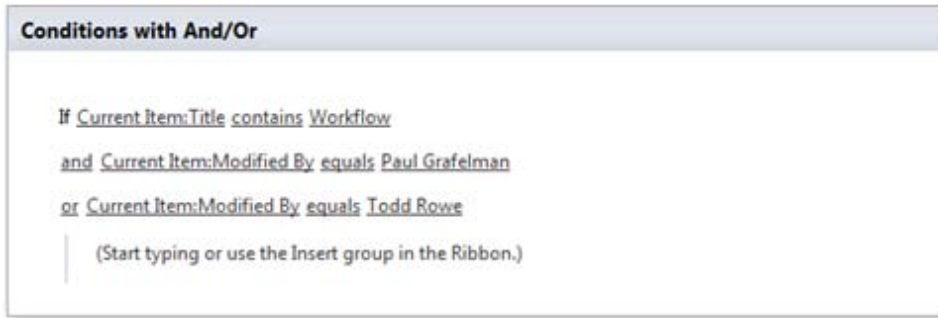
Figure 3.43 And and Or statements allow for multiple comparisons within one condition. This will allow you to create a single complex If statement instead of several simple If statements.
